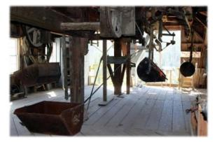
The principle of the tram system is relatively simple. The bucket was designed with Double Trucks (4-wheels) which rode over a large steel cable called the Stationary Cable. Each bucket was pulled along by another cable called the Traction Rope. The bucket was attached to the traction rope with a gripper, which automatically "gripped" and self-gripped itself as it entered or left the Tramhouse.
