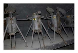
solution form, the first step of eliminating water was putting them in the presses. With most of the water now pressed out but still damp, the samples were spread out in trays and completely dried in the ovens in the adjacent room. There they would be split and put in envelopes, half going to the Lab for assaying, the remainder kept as a backup.
