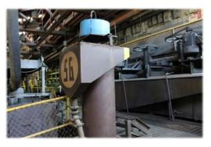
surface in the form of froth. Now separated, the copper mineral flowed up over the top of the pipe into the catch box. This concentrate was piped down to the Copper Filters for final treatment, while the Lead Mineral concentrate went to the Lead Thickener Tank to start the de-watering process.
