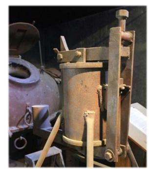
which forced the excess Mercury to pass through the filter and drop into a bucket of water. This procedure was called "Pressing Cakes", and took from 20 to 30 minutes. At this point the air was turned off and bled and the press opened up.
