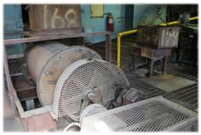
lbs. of Mercury was added, the amount determined by the ounces of Gold involved. This final mixture was again rotated for 3 hours but on a lower speed.
