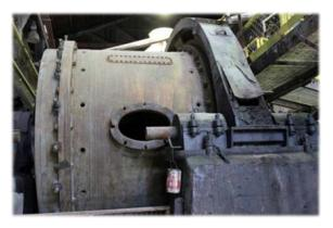
charged into the mill daily, rolling down through a pipe from the Ball Bins above. All of the material (Pulp) discharging from the mill would immediately enter the Gold Jigs (Station No.12).
