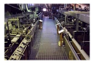
over into the front launder (trough) and was pumped to the Lead Cleaner Cells.
