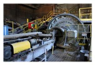
front of the mill to be discarded. In order to maintain the initial 48 tons of weight, 2 to 3 rods were charged into the mill daily.
