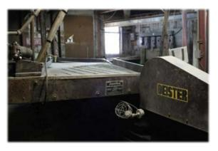
table, the Jig material immediately started spreading out over the surface. As the material began working its way over the riffles and towards the right hand end, the water washed the lighter particles over the bottom edge to be shipped back into the milling process.
