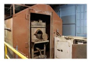
the furnace. As the contents became molten, they would separate themselves into different layers according to weight The Gold being the heaviest would go to the bottom. At a given temperature the door would be opened and the furnace rotated on the axle while pouring the layered molten material.
