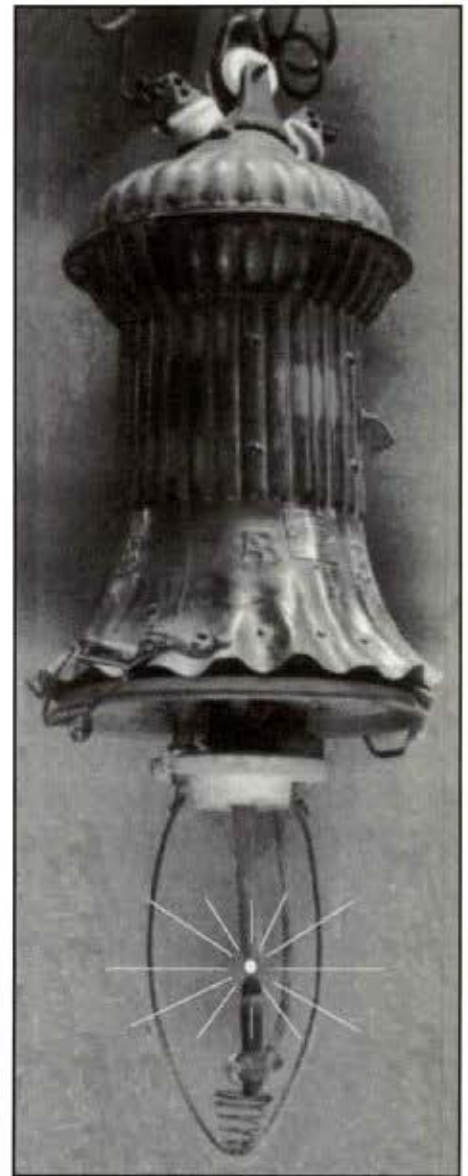
A carbon arc light fixture of the same type used in Aztec. They were in widespread use from 1895 until 1929.
